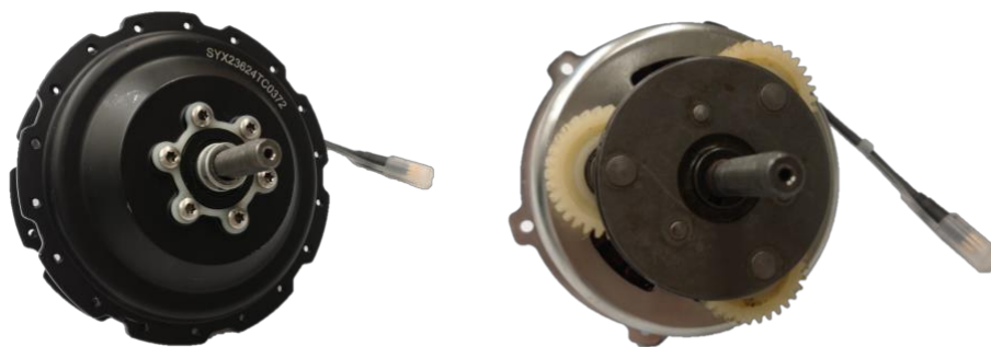
Figure 1: Image of the EBS SGI-G V2 motor in closed (left) and open (right) state
