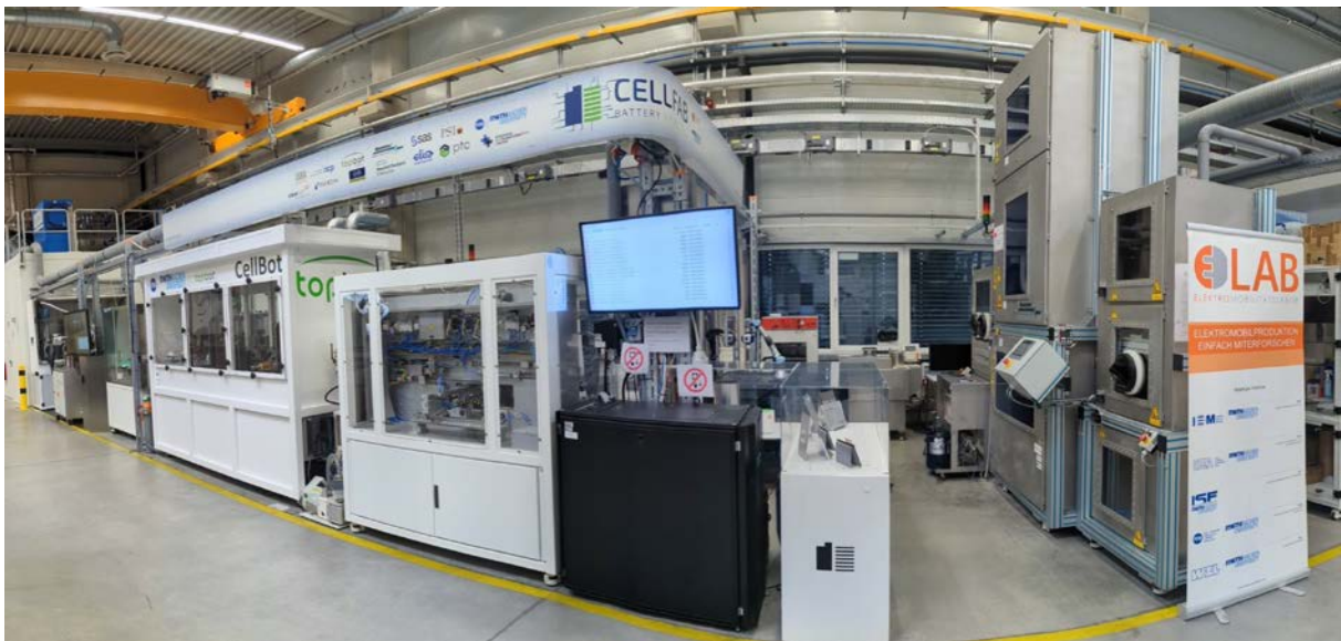
Figure 6: CELLFAB Battery Cell Production Line at PEM of RWTH Aachen University
