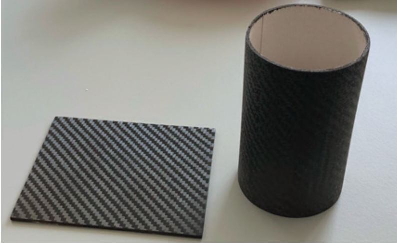
Figure 3: Hybrid Carbon fiber and ceramic material.
