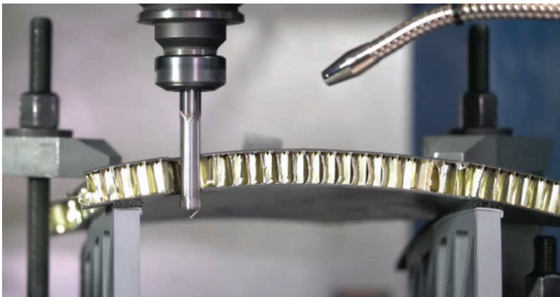
Figure 3: Typical processing situation of a CFRP-aluminium sandwich material.
